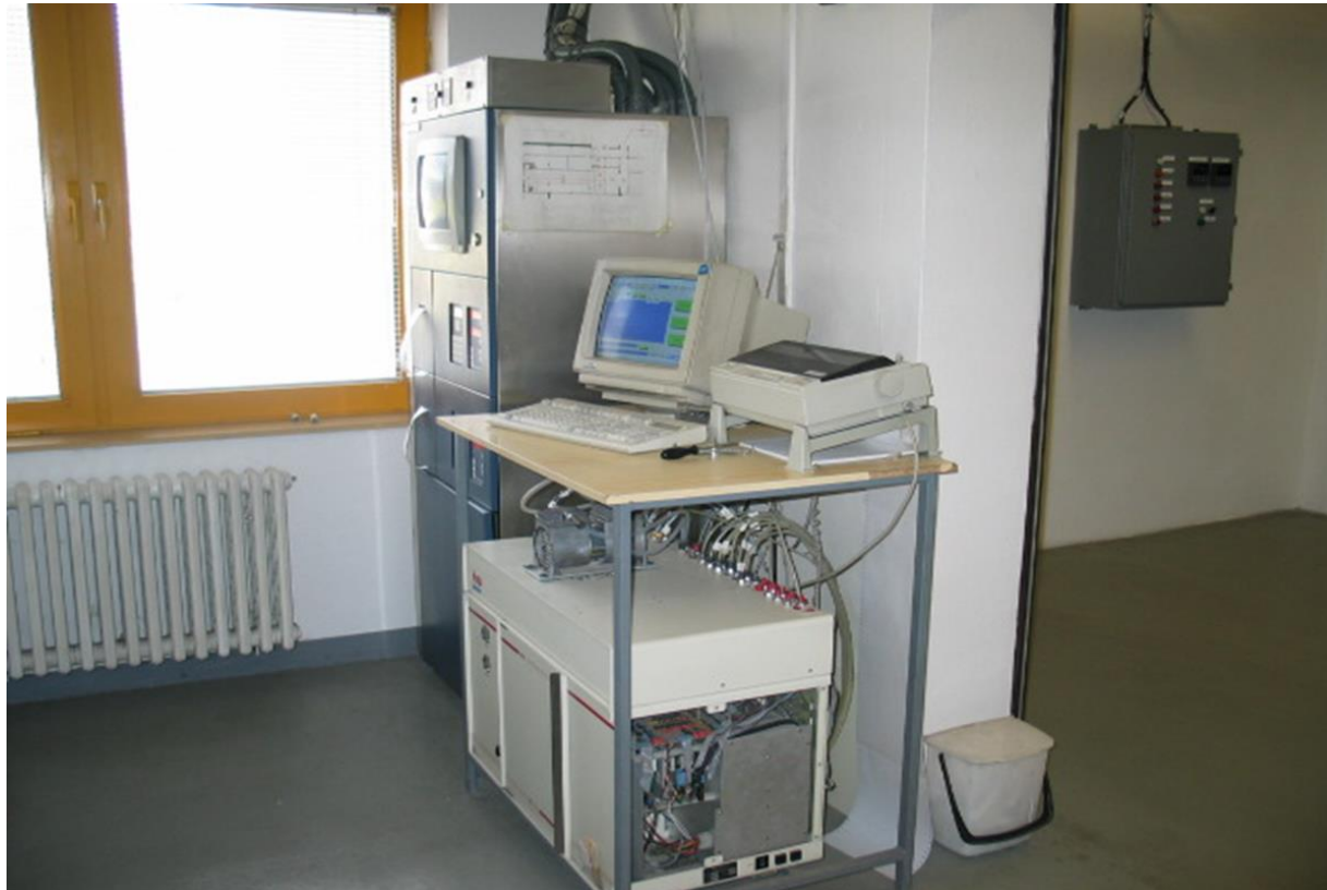
Controlling computer and gas chromatograph
